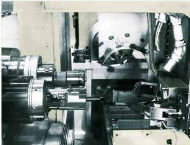
**CYLINDER BLOCK** Deep Hole Drilling
