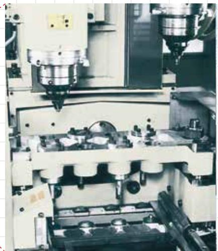
**CYLINDER BLOCK** Line Boring ATC
