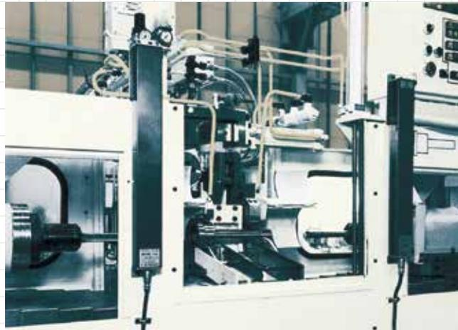
**CYLINDER BLOCK** Line Boring Auto Compensation
